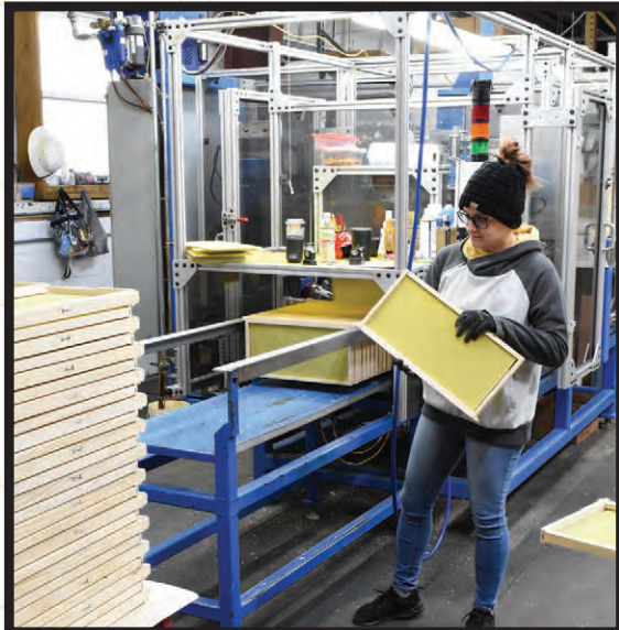
Machine to manufacture assembled frames with foundation at our Hamilton, IL. location. Each frame is secured by ample amounts of glue along with heavy duty staples to hold frame structure.
