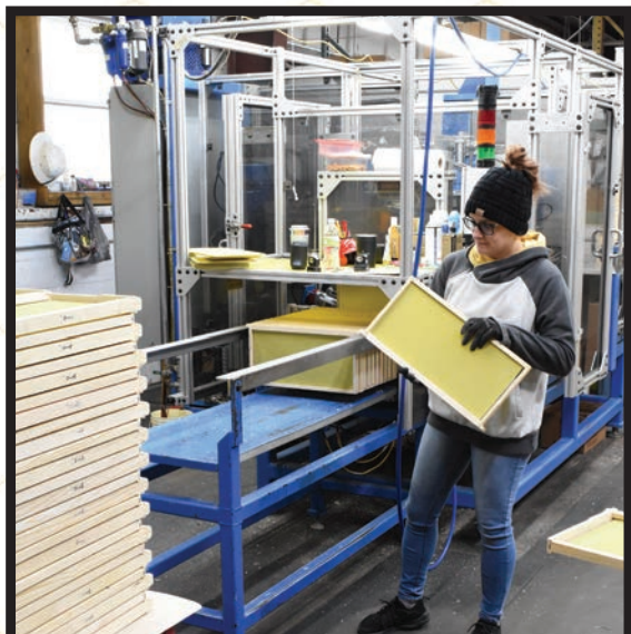
Machine to manufacture assembled frames with foundation at our Hamilton, IL. location. Each frame is secured by ample amounts of glue along with heavy duty staples to hold frame structure.
