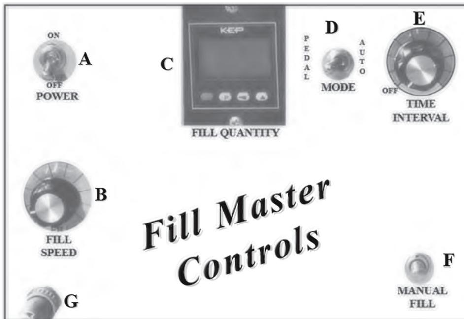
**A. Power Switch** - Turns the entire unit “on” and “off”. The filler can always be stopped from filling by turning this switch “off”.
